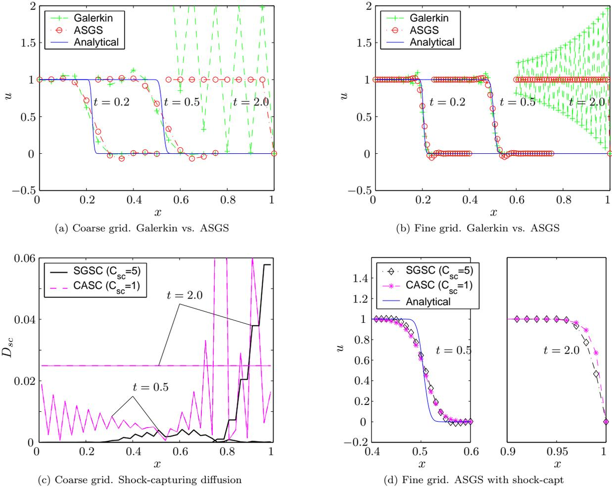
Figure 4: 1D miscible flow with zero distributed sources. ASGS vs. Galerkin solution and ASGS with shock-capturing at three different times, for a very coarse (left) and a finer (right) discretization
