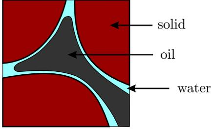
Figure 3: Schematic of immiscible flow of two fluid phases
