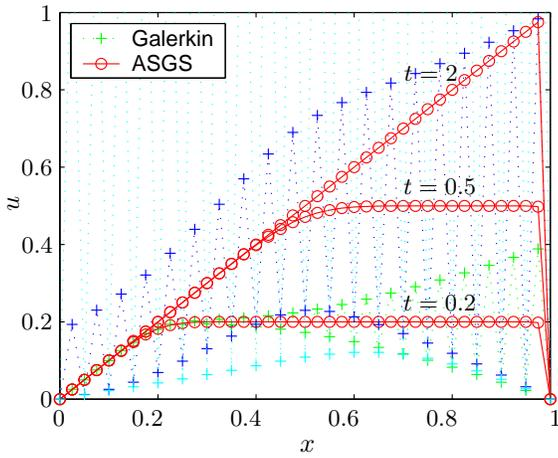
Figure 6: 1D miscible flow with nonzero distributed sources. ASGS vs. Galerkin solution at three different times
