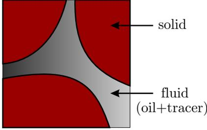
Figure 2: Schematic of miscible flow of two components in a single fluid phase
