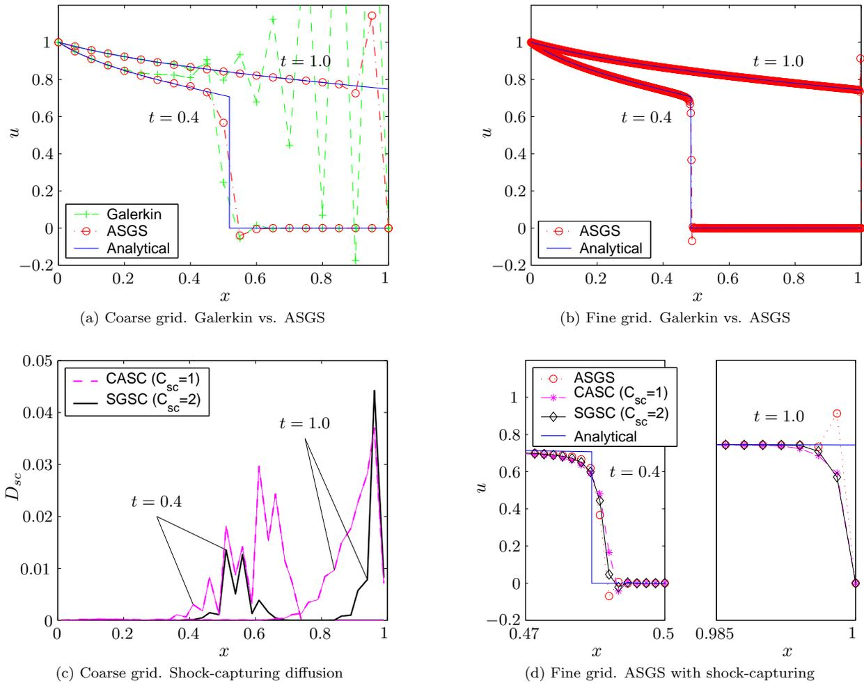
Figure 10: 1D immiscible flow. ASGS vs. Galerkin solution and ASGS with shock-capturing at two different times, for a very coarse (left) and a fine (right) discretization
