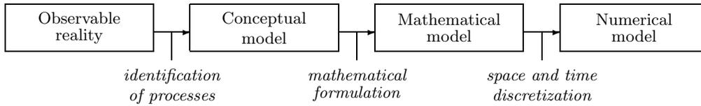
Figure 1: Steps in the development of a numerical model
