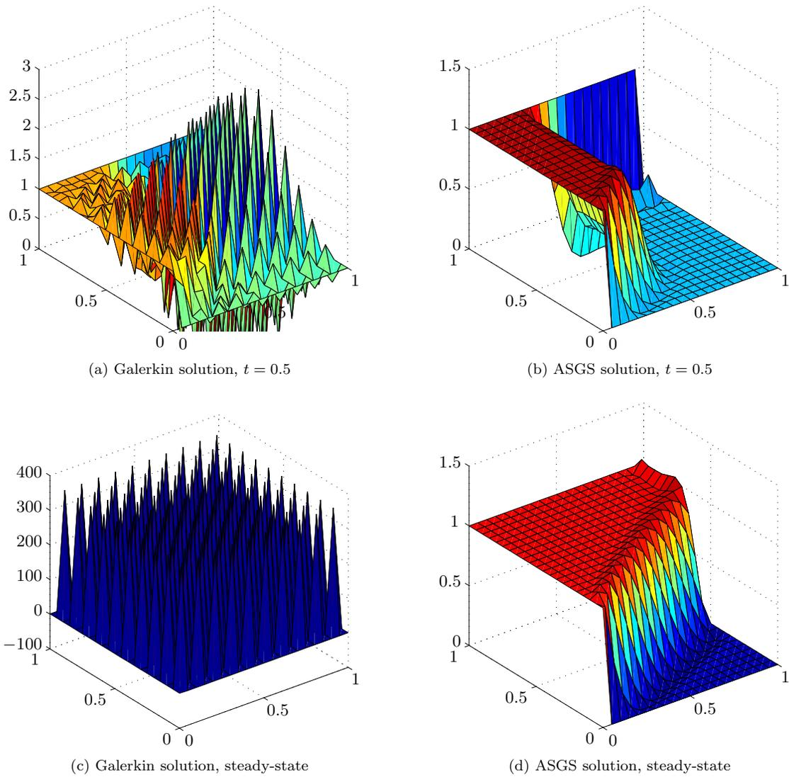
Figure 8: 2D miscible flow. Galerkin and ASGS solutions for transient and steady-state conditions
