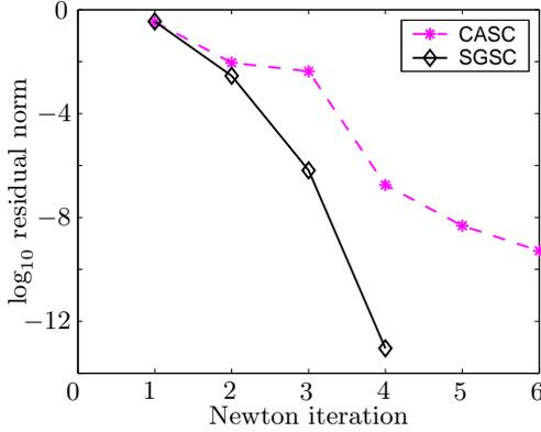
Figure 5: 1D miscible flow with zero distributed sources. Convergence of the ASGS method with shock-capturing at  $t = 0.5$
