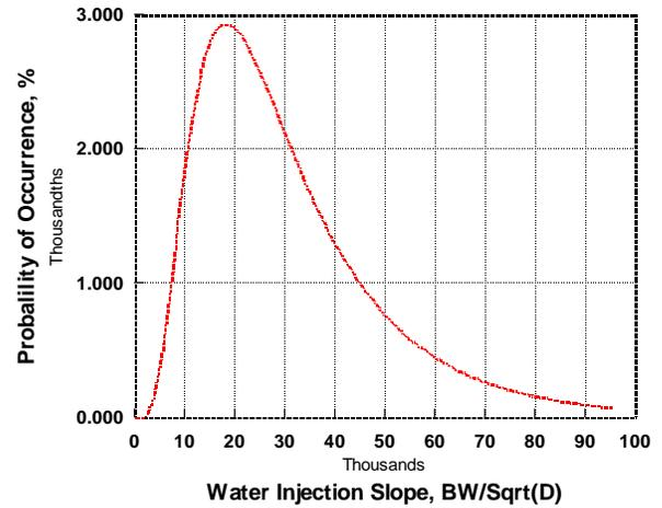
Fig. 21—The lognormal distribution of water injection slopes at Dow-Chanslor. The distribution mode is 18,600, its median is 28,700, and the mean is 32,300 BW per square root of days on injection. The mean plus three standard deviations (99.7% of all wells) is less than 97,000 BW/Sqrt(D).
