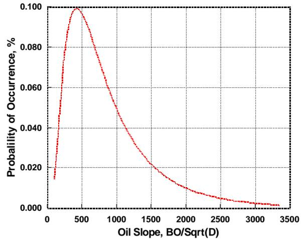
Fig. 17—The lognormal distribution of oil production slopes at Dow-Chanslor. The distribution mode is 420, median is 717 and mean is 937 BO per square root of days on production. The mean plus three standard deviations (99.7% of all wells) is below 3300 BO/Sqrt(D).
