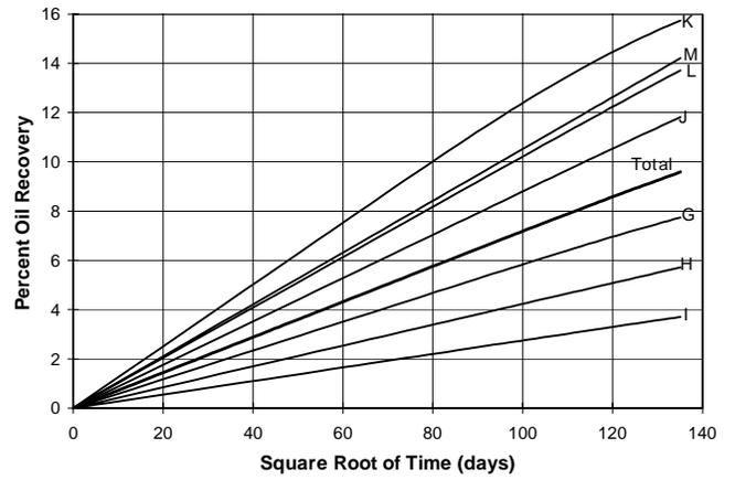
Fig. 8—Percent oil recovery in each layer. No infill or injection.
