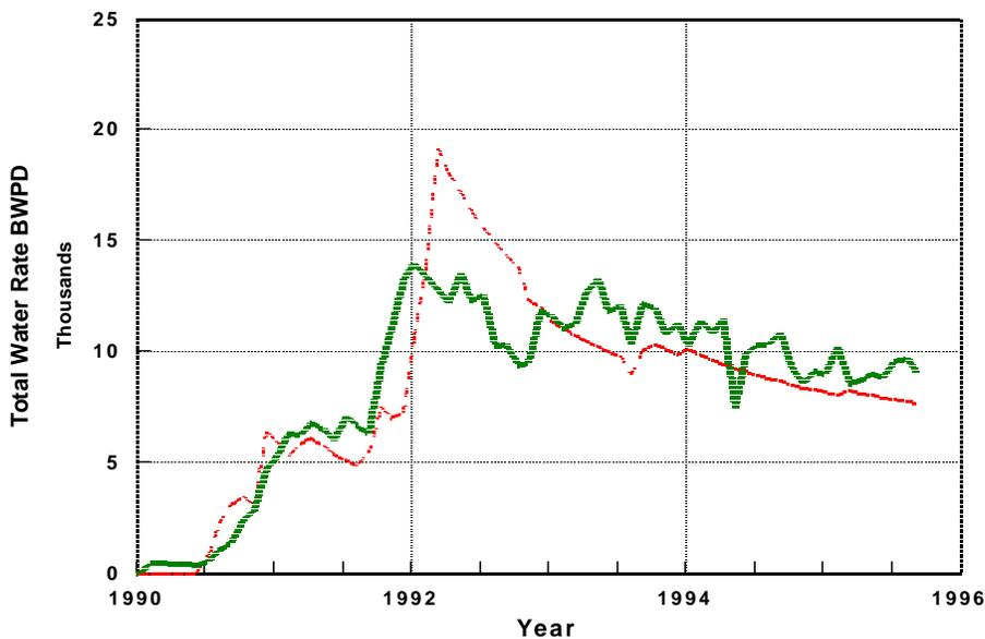
Fig. 23—The actual (solid line) and predicted (broken line) water injection at the Dow-Chanslor Fee, Section 1. Note that the model prediction can be run into the future and additional infill wells can be added, resulting in a reasonably good water injection forecast.
