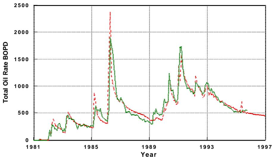
Fig. 22—The actual (solid line) and predicted (broken line) oil production at the Dow-Chanslor Fee, Section 1. Note that the model prediction can be run into the future and additional infill wells can be added, resulting in a very good oil production forecast.
