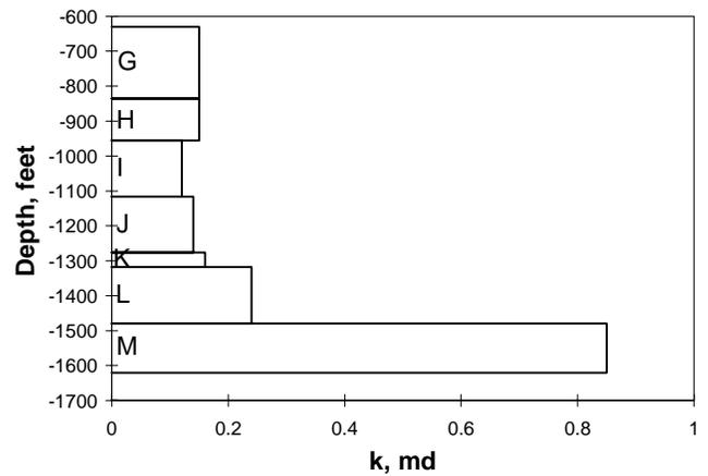
Fig. 4—Average diatomite layer permeability in millidarcies as a function of depth.
