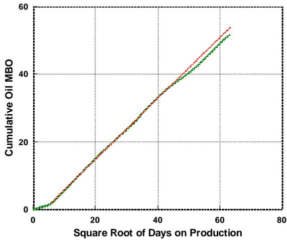
Fig. 14—Cumulative oil production from an average, time-shifted Crutcher-Tufts Section 1 well versus the square root of time. The average oil slope for 77 producers is 900 BO per square root of days on production. Note that only the oldest wells underperform the single trend above.
