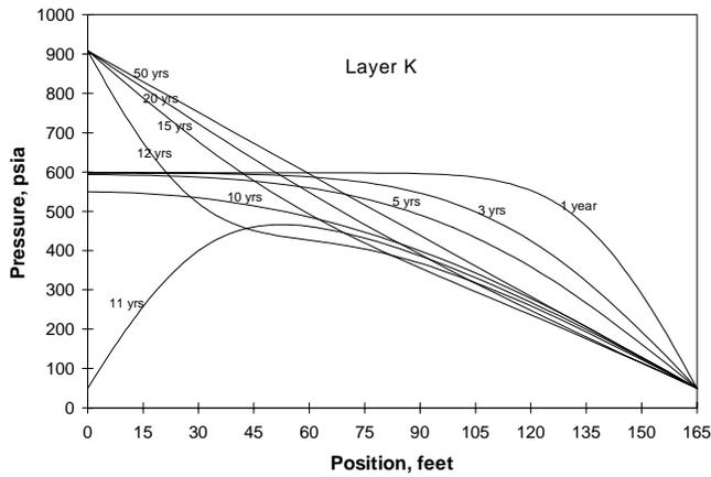
Fig. 9c—Pressure in layer K, psia, versus the position from infill well, feet. Infill at 10 years and injection at 11 years.
