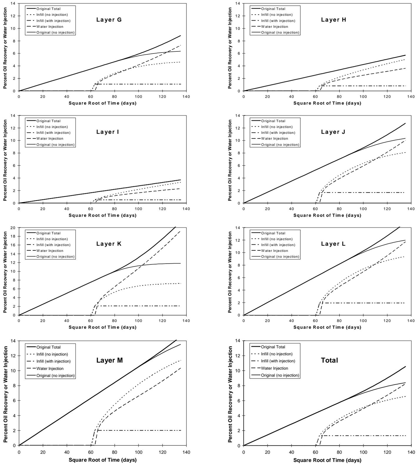
Fig. 10—Percent oil recovery or water injection versus the square root of time, days<sup>1/2</sup>, calculated as the amount produced or injected divided by the original-oil-in-place times 100 percent. Infill at 10 years and injection at 11 years.
