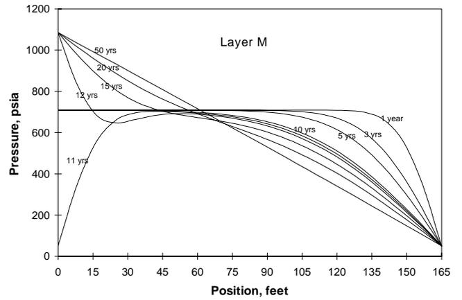
Fig. 9d—Pressure in layer M, psia, versus the position from infill well, feet. Infill at 10 years and injection at 11 years.
