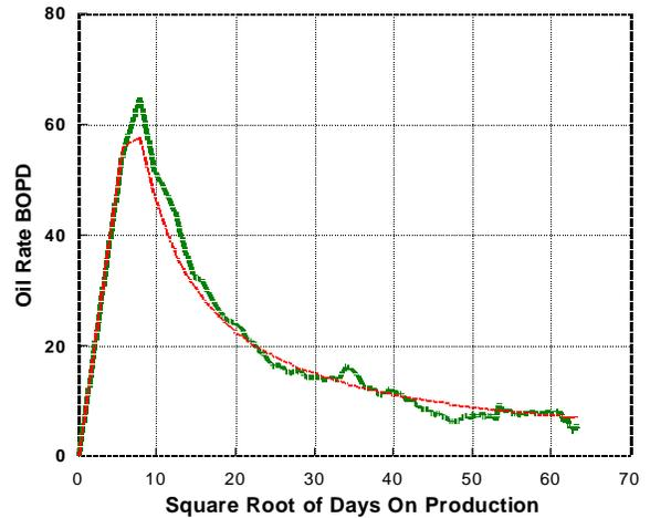
Fig. 15—Oil production rate from an average, time-shifted Crutcher-Tufts Section 1 well versus the square root of time. This is the oil rate expected from an average well in Section 1. Note a 100-day “startup-period.”
