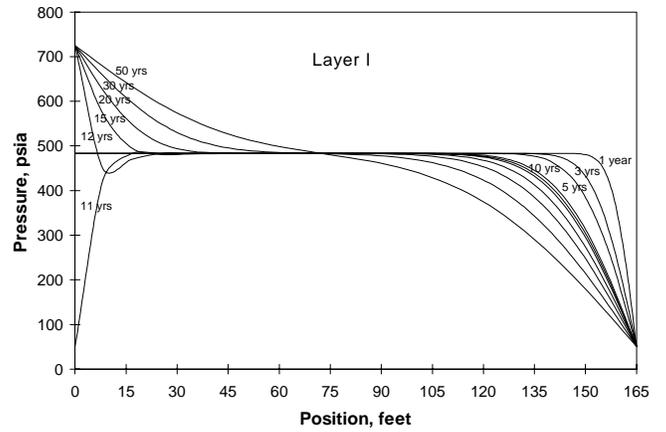
Fig. 9b—Pressure in layer I, psia, versus the position from infill well, feet. Infill at 10 years and injection at 11 years.
