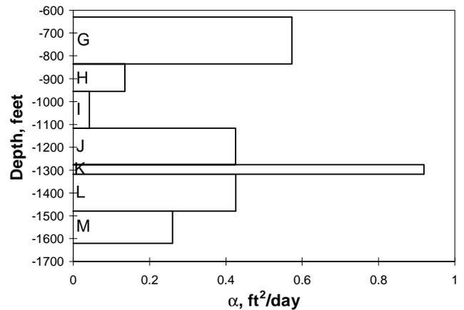
Fig. 6—Calculated  $\alpha$  in  $\text{ft}^2/\text{day}$  for the diatomite layers.
