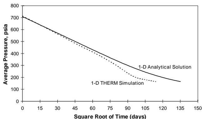
Fig. 12—Comparison of THERM simulation and analytical solution. Average layer pressure on primary for 50 years.
