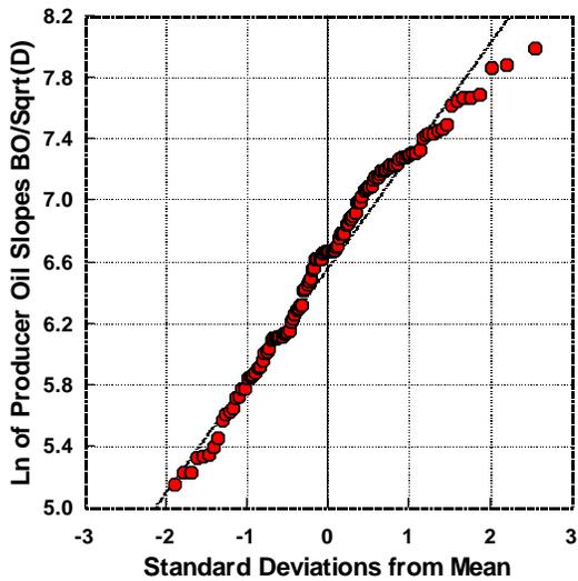
Fig. 16—Order statistics for 121 producers in the Dow-Chanslor Section 1 and 12 prove that their “oil slopes” are lognormally distributed. The intercept of the solid line is the mean and its slope is the standard deviation of the underlying normal population of the oil slope logarithms. Note the excellent fit.
