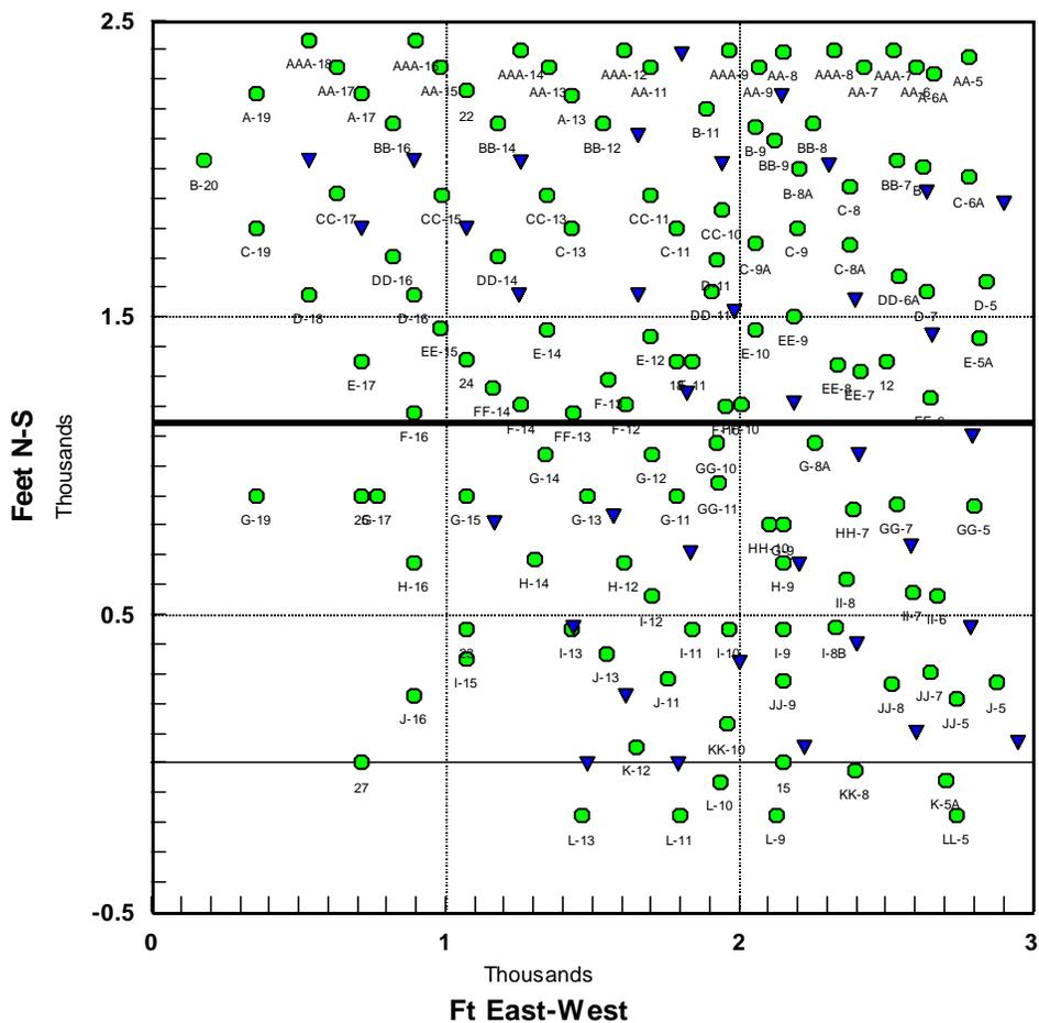
Fig. 13—The Crutcher-Tufts waterflood project in Sections 1 (the upper half) and 12 of the Dow-Chanslor Fee, Middle Belridge Diatomite, Kern County, CA. The triangles are water injectors.
