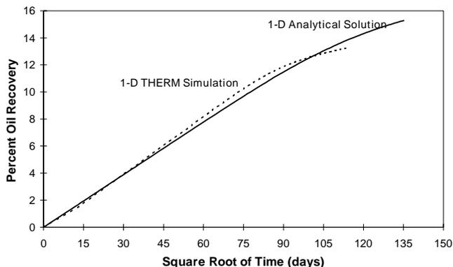
Fig. 11—Comparison of THERM simulation and analytical solution. Percent oil recovery on primary for 50 years.
