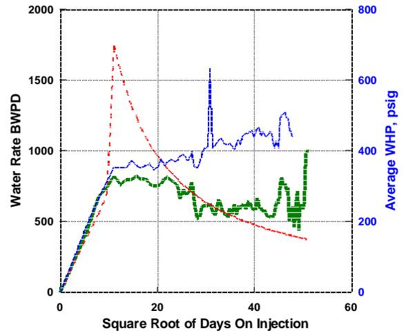
Fig. 19—Water injection rate and pressure (uppermost curve) in an average, time-shifted Crutcher-Tufts Section 1 well versus the square root of time. This is the water injection rate expected from an average well in Section 1, provided that the injection pressure is constant and there is no upper rate limit at early times. Note a 100-day “startup-period.”
