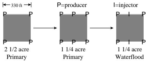
Fig. 1—Schematic of 2 1/2 acre primary followed by infill to 1 1/4 acres followed by conversion to water injection.
