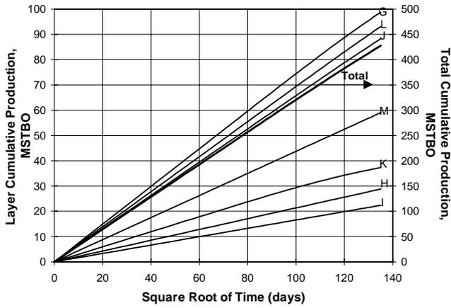
Fig. 7—Cumulative oil production in each layer. No infill or injection.
