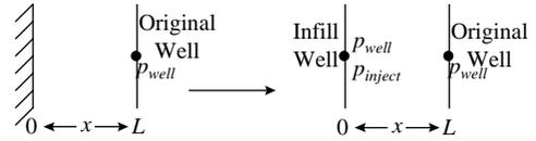
Fig. 2—Schematic for mathematical problem describing primary production followed by infill. Note the symmetry in the primary production at  $x = 0$  leads to a no flow boundary. The wells are prescribed pressure boundaries.
