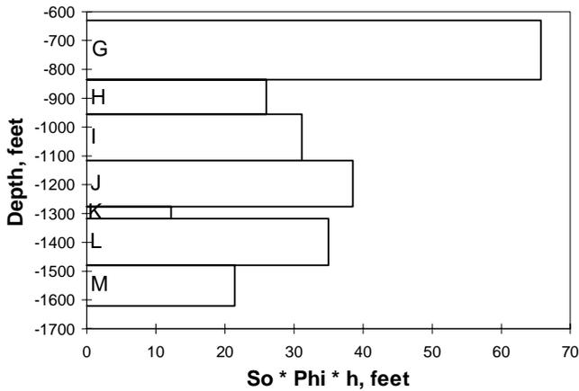
Fig. 3—Amount of oil per unit area of reservoir in each layer.
