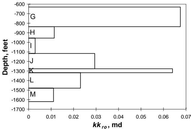
Fig. 5—Actual oil permeability in millidarcies for the diatomite layers.
