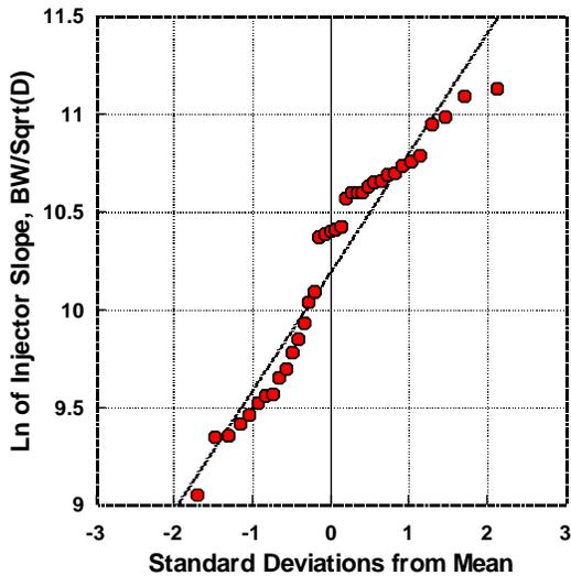
Fig. 20—Order statistics for 37 water injectors in Section 1 and 12 of Dow-Chanslor. The population of “water slopes” is not homogeneous and there seem to be 2-3 underlying sub-populations. Nevertheless, the water slopes are lognormally distributed.
