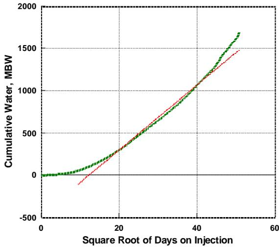
Fig. 18—Cumulative water injection in an average, time-shifted Crutcher-Tufts Section 1 well versus the square root of time. The average water slope for 21 injectors is 34,500 BW per square root of days on injection. Note that the fit is not nearly as good as in Fig. 14 because of the average WHP increases with time.
