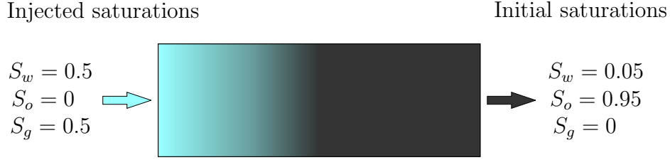
Figure 20. Sketch of the injection problem. Water and gas are injected into a core initially filled with oil and water.
