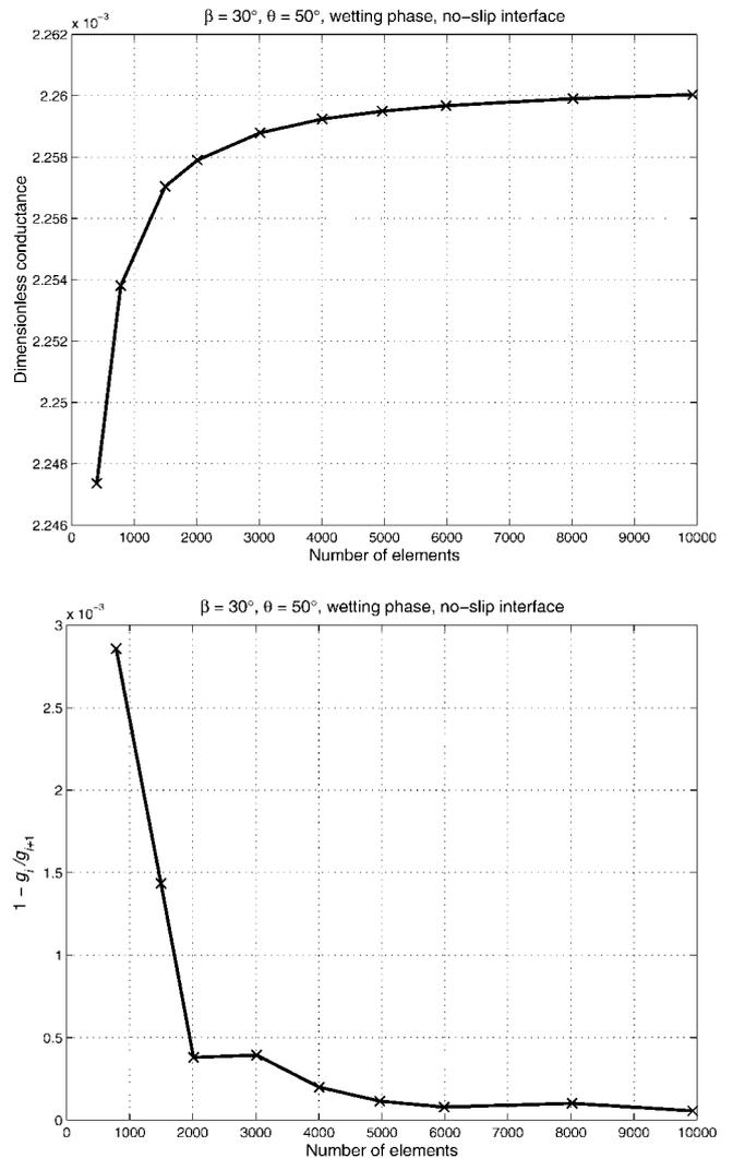
**FIG. 6.** Convergence of the FE solution for the wetting fluid hydraulic conductance in the perfectly rigid interface case.
