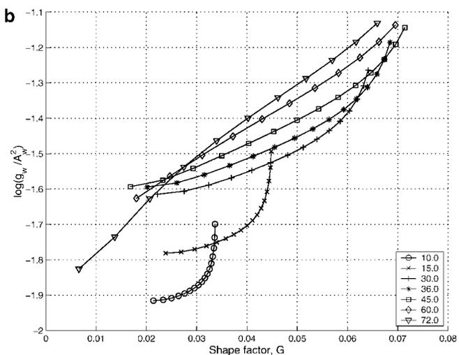
**FIG. 13.** (a) The logarithm of the dimensionless hydraulic conductance in the perfect-slip case vs. contact angle. (b) The logarithm of the ratio of the dimensionless hydraulic conductance and the dimensionless corner filament area squared plotted vs. the filament shape factor. The half-angles of the corners are between  $10^\circ$  and  $72^\circ$ .
