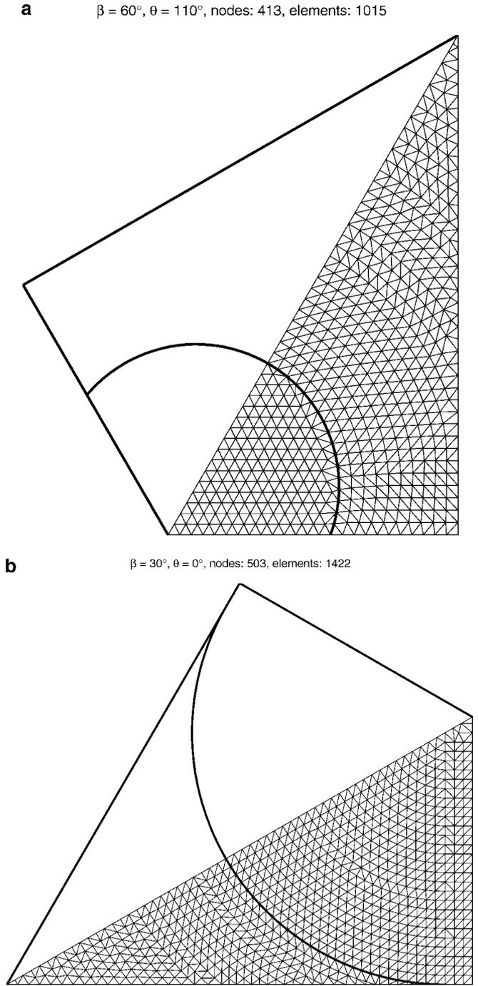
**FIG. 5.** Optimized finite element meshes for the corner half-angle of  $60^\circ$  and contact angle of  $110^\circ$  (a), and  $30^\circ$  and  $0^\circ$ , respectively, (b).
