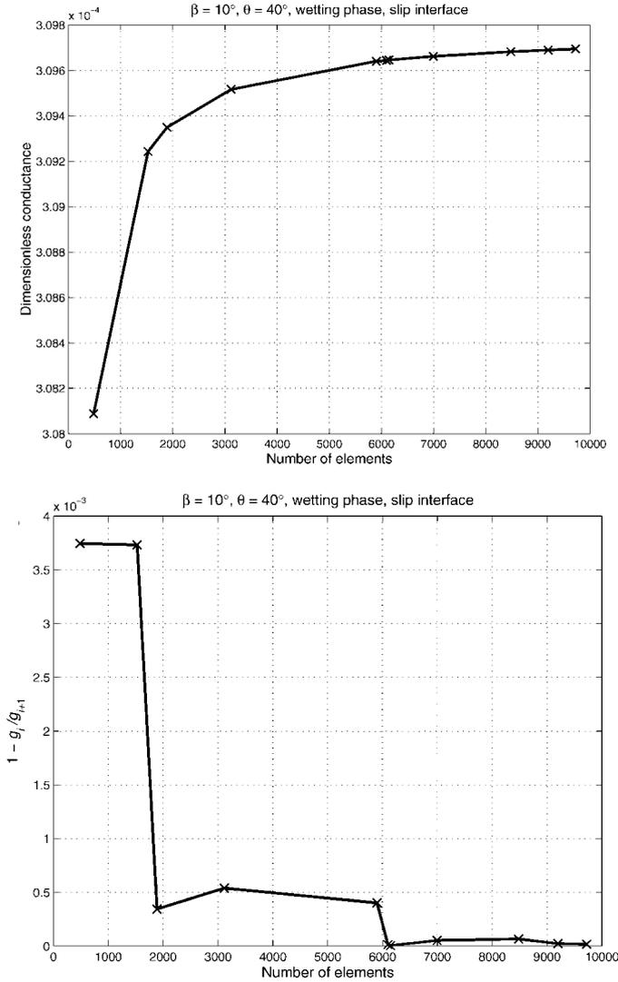
FIG. 7. Convergence of the FE solution for the wetting fluid hydraulic conductance in the perfect-slip interface case.
