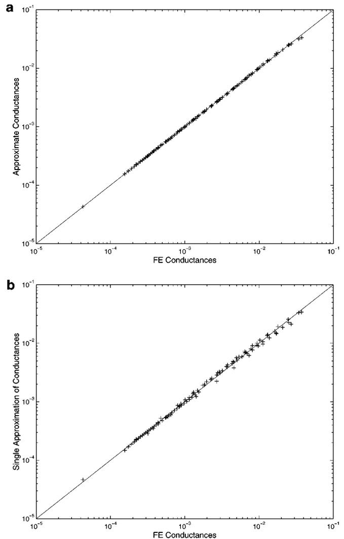
**FIG. 11.** Individual approximations for each corner half-angle (a) and a single approximation (b) for all corner half-angles versus the finite element results in the no-slip case.
