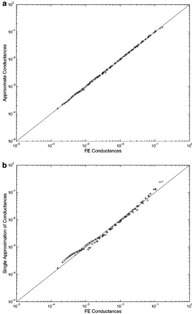
**FIG. 15.** Individual approximations for each corner half-angle (a) and a single approximation (b) for all corner half-angles versus the finite element results in the perfect-slip case.
