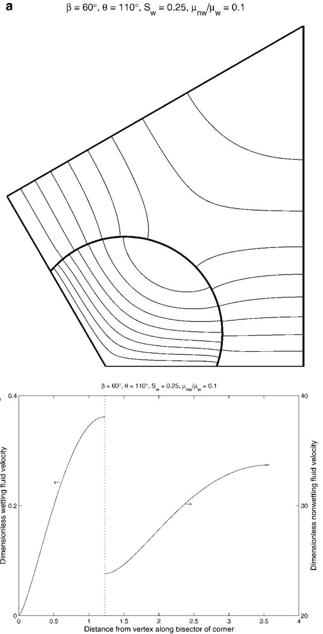
**FIG. 2.** Velocity distributions for the perfect-slip case. The corner half-angle is  $60^\circ$ , the contact angle is  $110^\circ$ , the wetting phase saturation is 0.25, and the nonwetting–wetting fluid viscosity ratio is 0.1: (a), velocity contours; (b), velocity profiles along the bisector of the corner angle, with the meniscus position highlighted by the vertical line.
