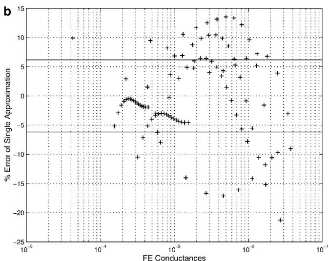
**FIG. 12.** The mean absolute error of the individual approximations (a) in the no-slip case is 1%, while that of the single approximation (b) is 6.2%.
