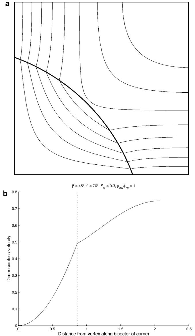
**FIG. 4.** Velocity distributions with continuity of velocity and shear stress across the interface. The corner half-angle is  $45^\circ$ , the contact angle is  $70^\circ$ , the wetting phase saturation is 0.30, and the nonwetting–wetting fluid viscosity ratio is 1: (a), velocity contours; (b), velocity profiles along the bisector of the corner angle, with the meniscus position highlighted by the vertical line.
