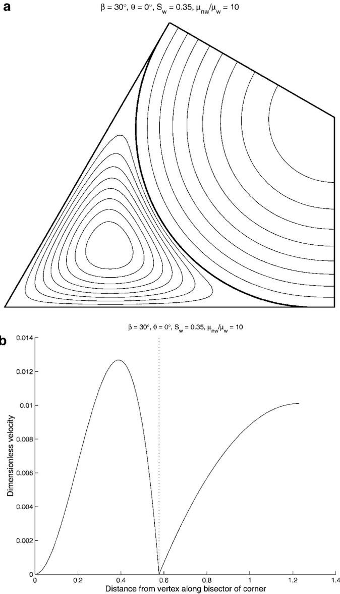
**FIG. 1.** Velocity distributions for the no-slip case. The corner half-angle is  $30^\circ$ , the contact angle is  $0^\circ$ , the wetting phase saturation is 0.35, and the nonwetting–wetting fluid viscosity ratio is 10: (a), velocity contours; (b), velocity profiles along the bisector of the corner angle, with the meniscus position highlighted by the vertical line.
