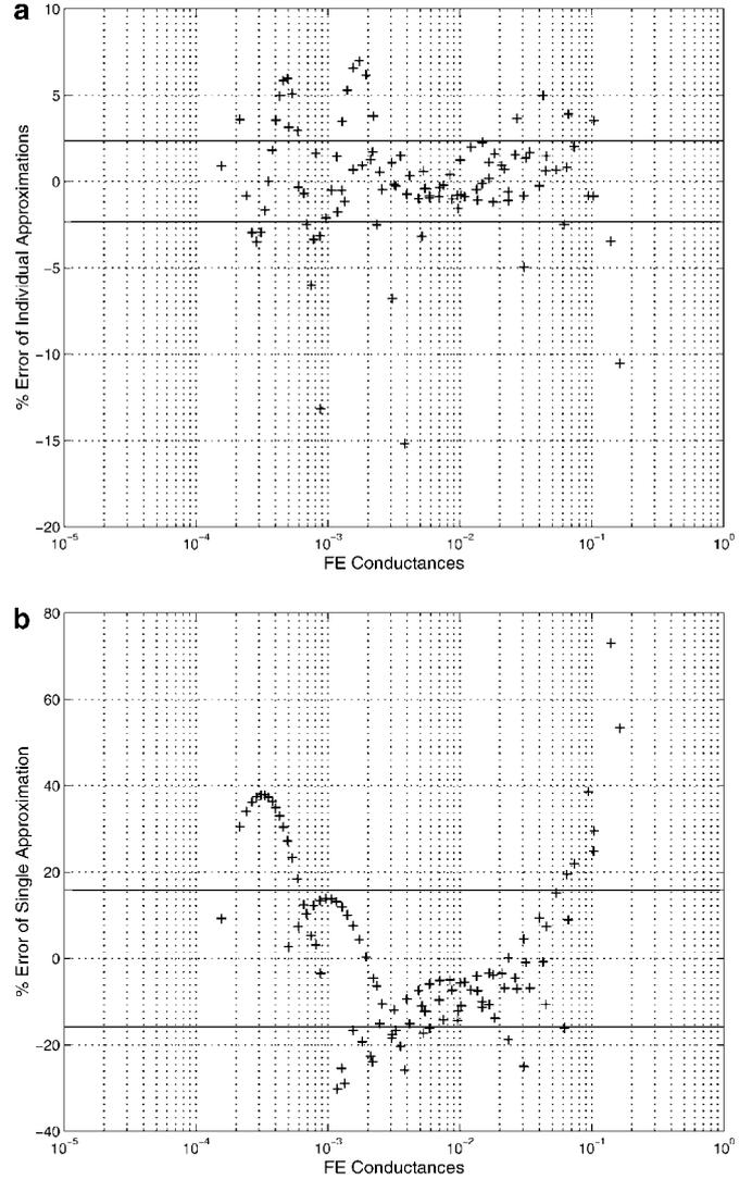
**FIG. 16.** The mean absolute error of the individual approximations (a) in the perfect-slip case is 2.2%, while that of the single approximation (b) is 15.9%.
