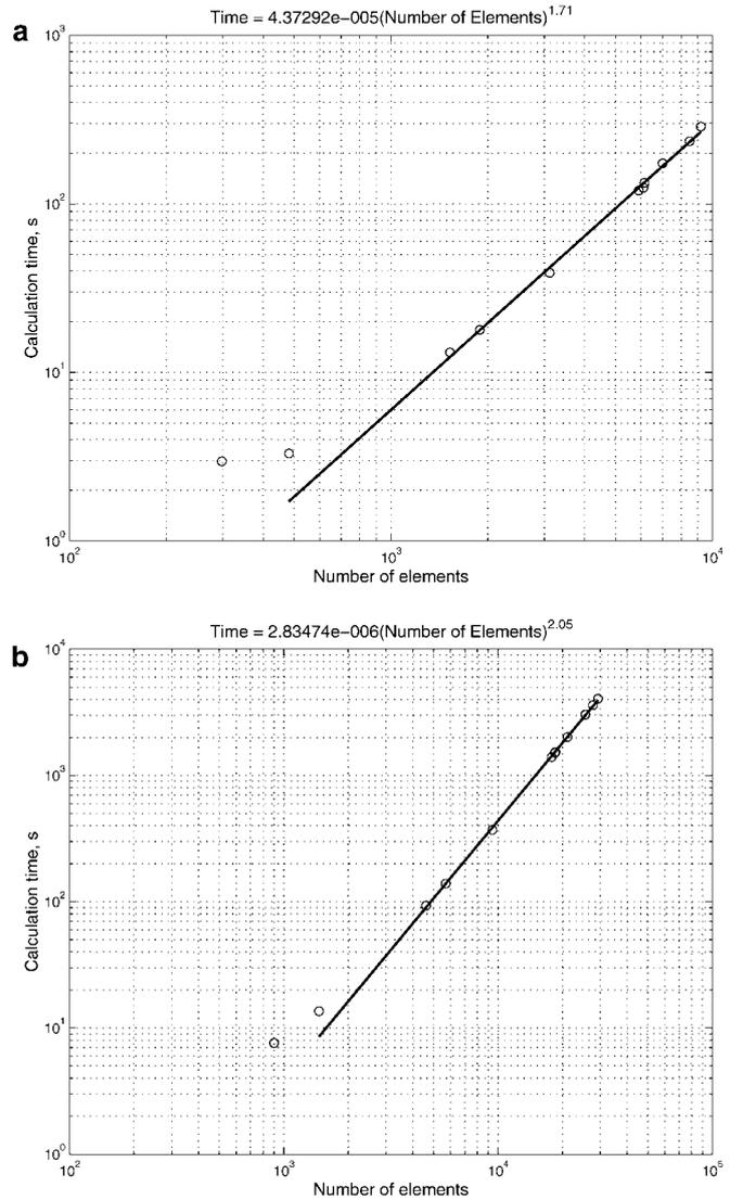
FIG. 8. (a) Calculation times for  $\beta = 10^\circ$ ,  $\theta = 40^\circ$ , no-slip boundary condition, and only wetting fluid domain. (b) Calculation times for  $\beta = 10^\circ$ ,  $\theta = 40^\circ$ , perfect-slip boundary condition, and both domains with  $S_w = 0.25$ .
