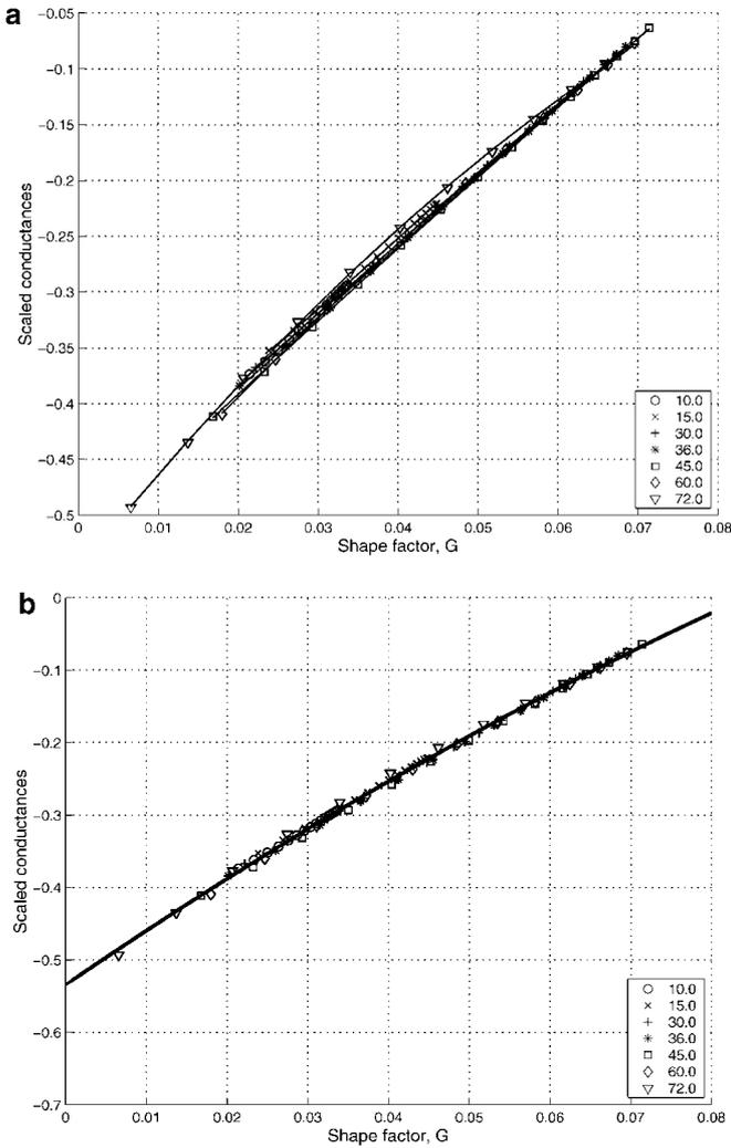
**FIG. 10.** The scaled hydraulic conductance approximations for each corner half-angle (a) and the single master curve (b) vs. the filament shape factor.
