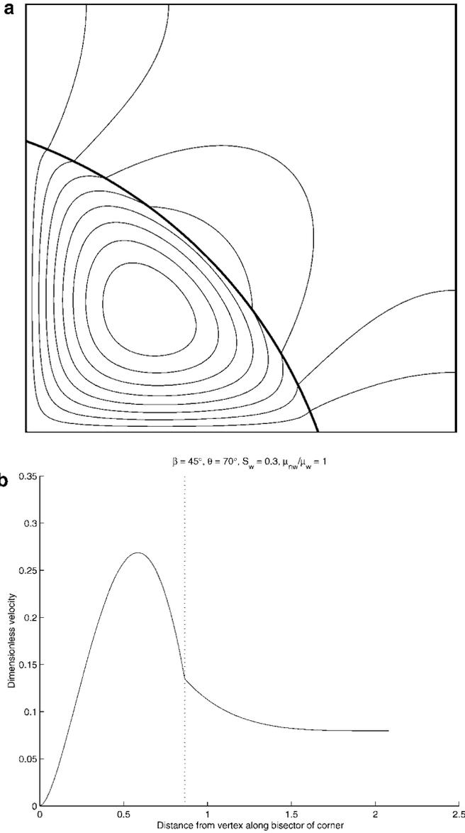
**FIG. 3.** Velocity distributions with continuity of velocity and shear stress across the interface. The corner half-angle is  $45^\circ$ , the contact angle is  $70^\circ$ , the wetting phase saturation is 0.30, and the nonwetting–wetting fluid viscosity ratio is 1: (a), velocity contours; (b), velocity profiles along the bisector of the corner angle, with the meniscus position highlighted by the vertical line.
