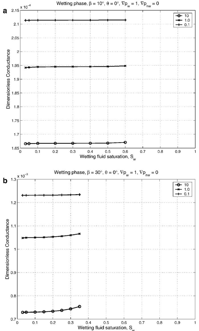
**FIG. 18.** The dimensionless hydraulic conductance in coupled flow of a perfectly wetting fluid as a function of the fluid saturation at three nonwetting-fluid viscosity ratios. The corner half-angles are  $10^\circ$  (a) and  $30^\circ$  (b).
