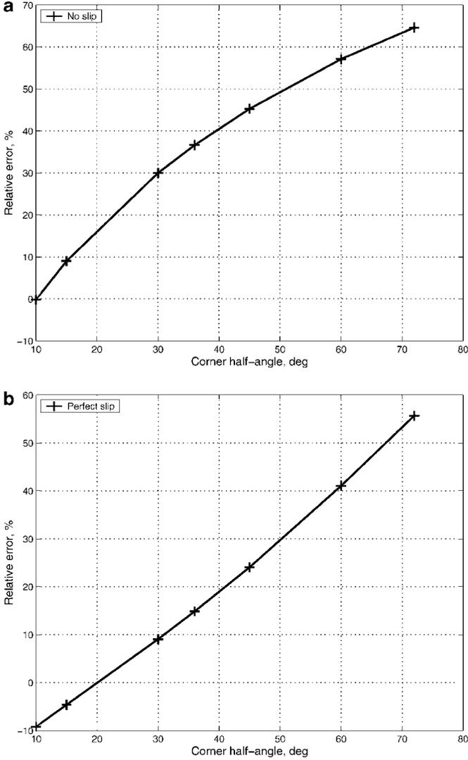
**FIG. 17.** Relative deviations of Zhou *et al.*'s analytical flow resistance factors from the corresponding FE solutions for zero contact angles: (a) no slip; (b) perfect slip.
