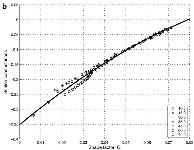
**FIG. 14.** The scaled hydraulic conductance approximations for each corner half-angle (a) and the single master curve (b) vs. the filament shape factor.
