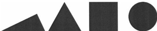
FIG. 2. Idealization of a pore body and the attached pore throats as cylinders of square and circular cross-sections.
