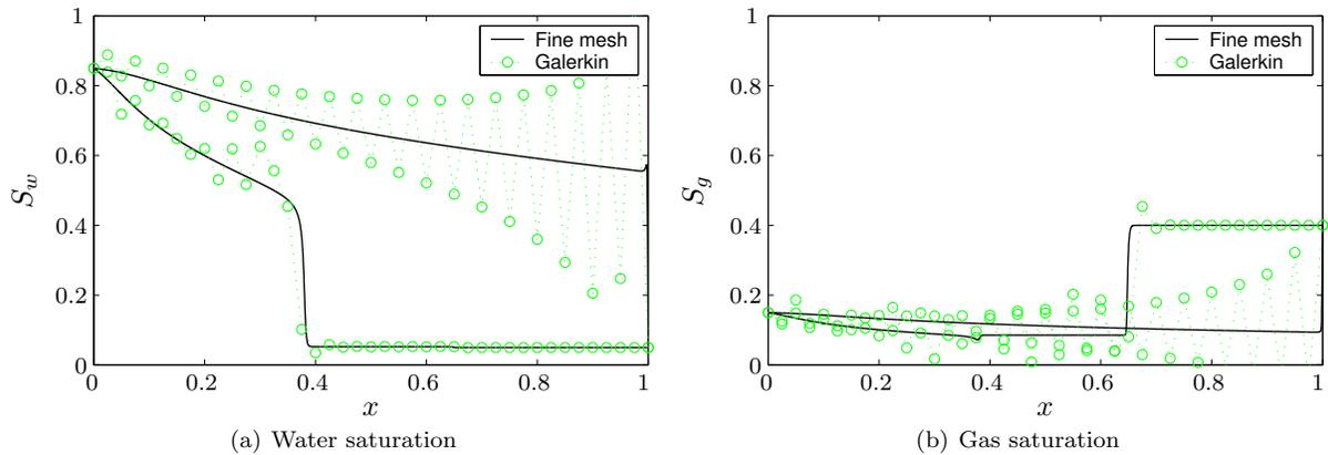
Fig. 16— Saturation profiles of the standard Galerkin solution to the water-gas injection problem on a coarse mesh of 40 elements. Results are shown at times  $t = 0.5$  and  $t = 2$ .
