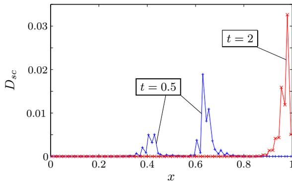
**Fig. 19— Profiles of shock capturing diffusion introduced by the proposed formulation at two different times.**
