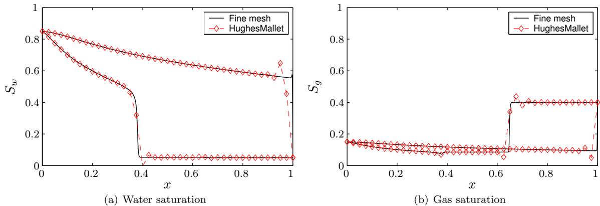
Fig. 17— Saturation profiles of the ASGS solution ( $\tau$  formulation given by Hughes and Mallet<sup>24</sup>) to the water-gas injection problem on the coarse mesh.
