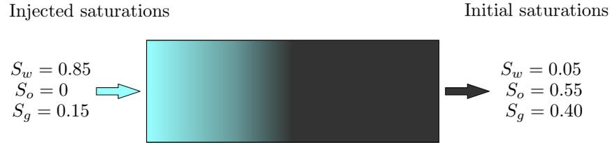
Fig. 12— Sketch of the water-gas injection problem. Water and gas are injected into a medium initially filled with oil and gas.
