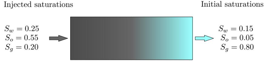
Fig. 1— Sketch of the oil filtration problem. A mixture with high oil saturation is injected into a relatively dry medium.
