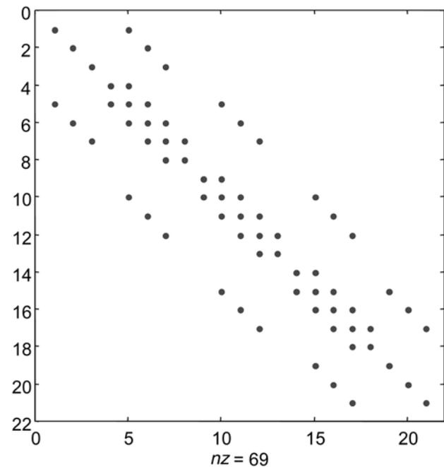
Fig. 5—The structure of the matrix  $[\Phi]^*[\mathbf{K}^1][\mathbf{B}][\Phi]$  on an irregular grid.
