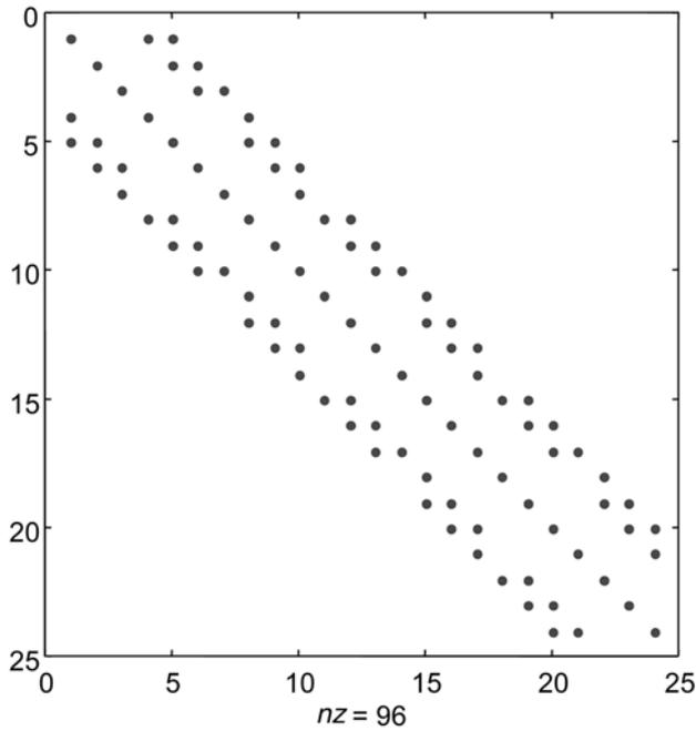
Fig. 3—The structure of the flux operator matrix on a rectangular grid. The  $x$  and  $y$  coordinates are the indices of the matrix elements. The elements that are nontrivial are denoted by dots; the zero elements are represented with spaces.
