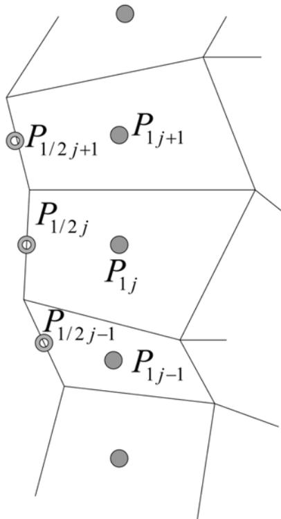
Fig. 1—Indexing of the interior and boundary cells.
