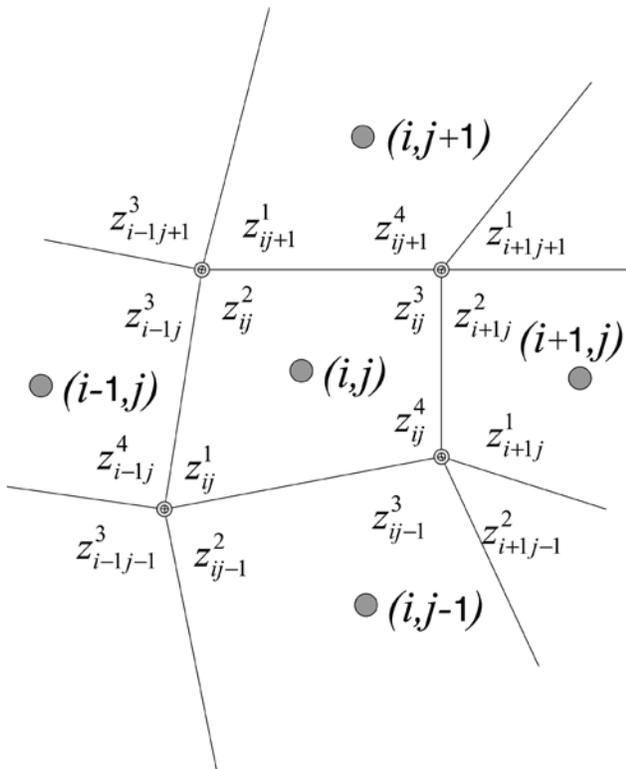
Fig. 10—The scalar function  $z$  may take up to four different values at each vertex of the cell  $(i,j)$ .
