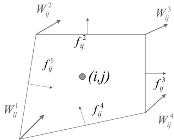
Fig. 2—Cell  $(i,j)$ :  $f_{ij}^{1,2,3,4}$  are the normal components of the fluxes attached to the walls of the cell, while  $w_{ij}^{1,2,3,4}$  are the fluxes at the corners of the cell.
