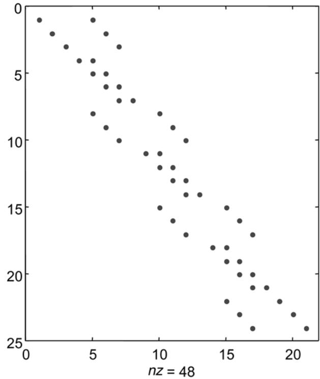
Fig. 4—The structure of discretized Laplace operator  $\nabla \cdot (\vec{k} \nabla p)$  on a rectangular grid. As in Fig. 3, the  $x$  and  $y$  coordinates are the indices of the matrix elements. The elements that are nontrivial are denoted by dots; the zero elements are represented with spaces.
