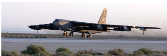
Figure 2. A B-52 Stratofortress takes off from Runway 22 during a FT test flight from Edwards Air Force Base, California, on Sept. 19, 2006. During the flight, two of the aircraft's eight engines ran on the natural gas-based FT fuel blend. The bombers are from the 5th Bomb Wing at Minot Air Force Base, N.D. (U.S. Air Force photo/Chad Bellay).
