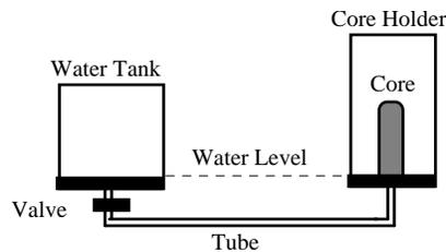
**Fig. 2 - Schematic of CT Scan Experiment**
