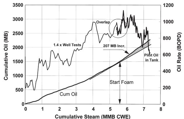
Fig. 8—Oil rate and cumulative oil produced in the Dome-Tumbador pilot vs. cumulative injected steam.
