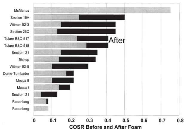
**Fig. 9—Cumulative oil steam ratio just before and after injection of steam foam.**
