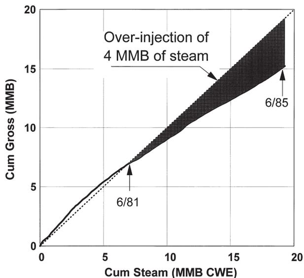
Fig. 6—Cumulative gross production in the Dome-Tumbador pilot vs. steam injection.
