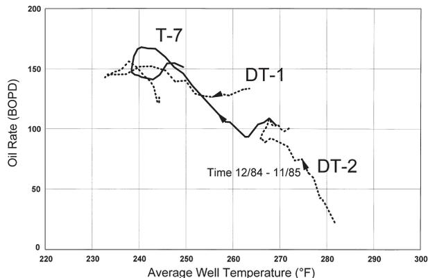
Fig. 3—Oil production vs. average BHT in three Dome-Tumbador wells follow an identical trend for almost 2 years.
