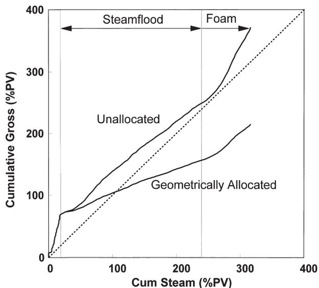
Fig. 4—Cumulative gross production in the Mecca steam-foam pilot vs. steam injection.
