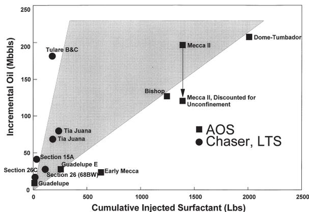
**Fig. 10—Cumulative incremental oil vs. cumulative injected mass of surfactant.**
