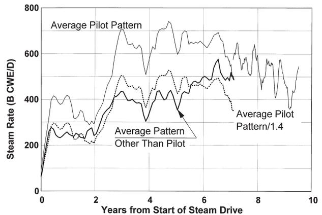
Fig. 7—Average steam injection rate per pattern in the Dome-Tumbador pilot and the nonpilot patterns.
