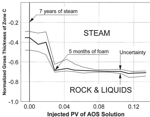
Fig. 1—A doubling of vertical sweep by steam foam in the Dome-Tumbador pilot.
