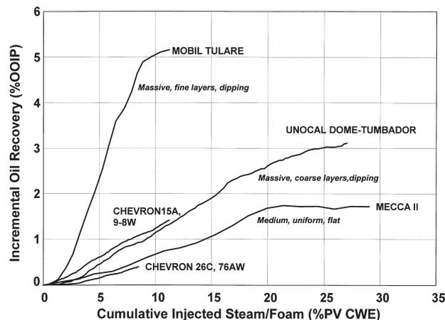
Fig. 2—Early production responses in several steam-foam pilots were almost instantaneous.
