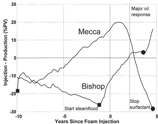
Fig. 5—Net liquid balance (Injection/gross production) for the Bishop and Mecca pilots.
