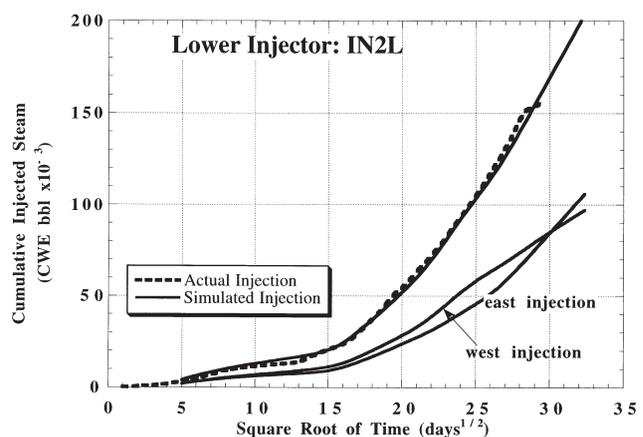
Fig. 4—Steam injection in IN2L, including injection to the east and west halves of the pilot.
