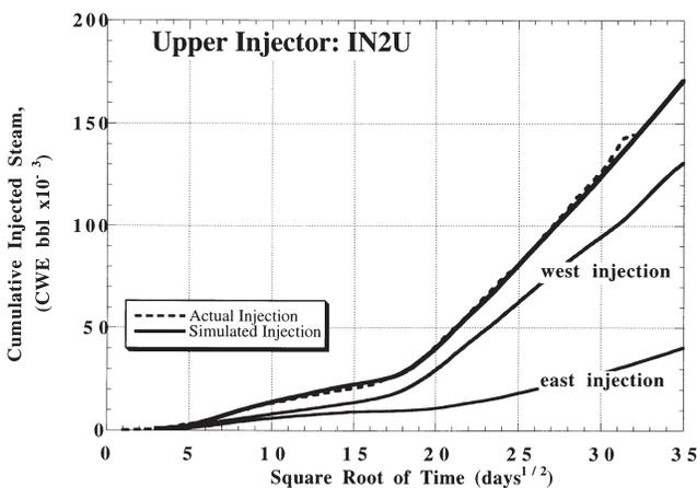
Fig. 3—Steam injection in IN2U, including injection to the east and west halves of the pilot.
