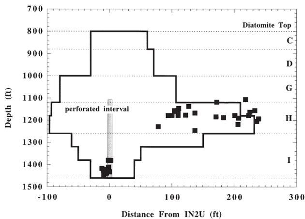
Fig. 9—Comparison between IN2U fracture shape from history matching and microseismic events.
