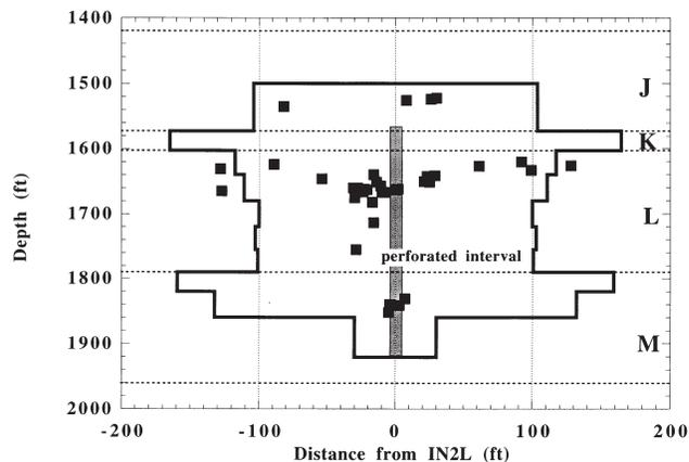
Fig. 10—Comparison between IN2L fracture shape from history matching and microseismic events.
