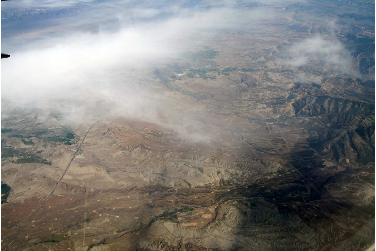
Figure 11: How is gas production kept relatively constant in the U.S.? By drilling a myriad of deep expensive gas wells, some of which were photographed by Patzek when he was flying over Colorado in the summer of 2007. In 2006, \sim 3,800 wells/month were drilled in the U.S., most of them for gas. Many of the new gas wells decline initially at 33% per year in the first 1 – 2 years, switching to the low production regime later. Image source: T. W. Patzek.
