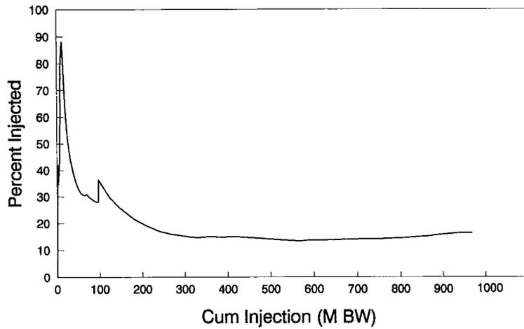
Fig. 13—Water produced by the Phase I “High Gross” wells as percent of cumulative injection in the “High Rate” injectors. Note the severe imbalance, suggestive of fracture extension and reservoir damage.
