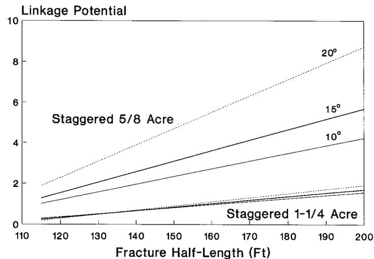
Fig. 3b—Dimensionless linkage potential for ½- and 1¼-acre (0.25- and 0.5-ha) staggered line patterns.
