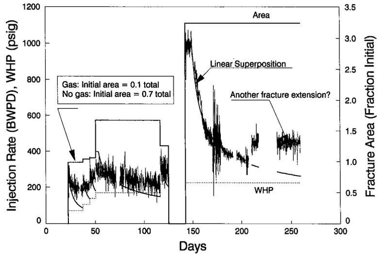
Fig. 24—Injection rate and fracture extensions during four pressure steps in Phase I injector 555E-33. Note that in the worst case the fracture area could be twice the design area.
