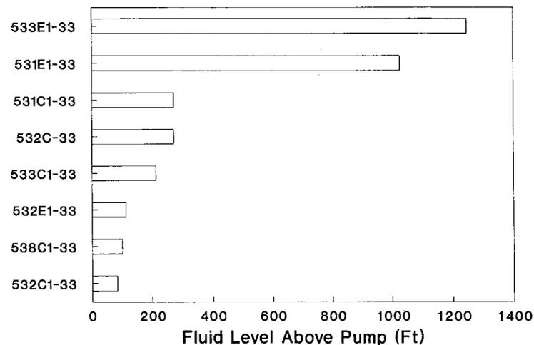
Fig. 18—Fluid levels in the high-gross producers in the seven-pattern, 1/4-acre waterflood pilot.
