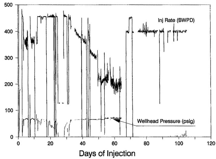
Fig. 21—Injector 538A-28 links with 531E1-33 after 62 days of injection and goes on vacuum.
