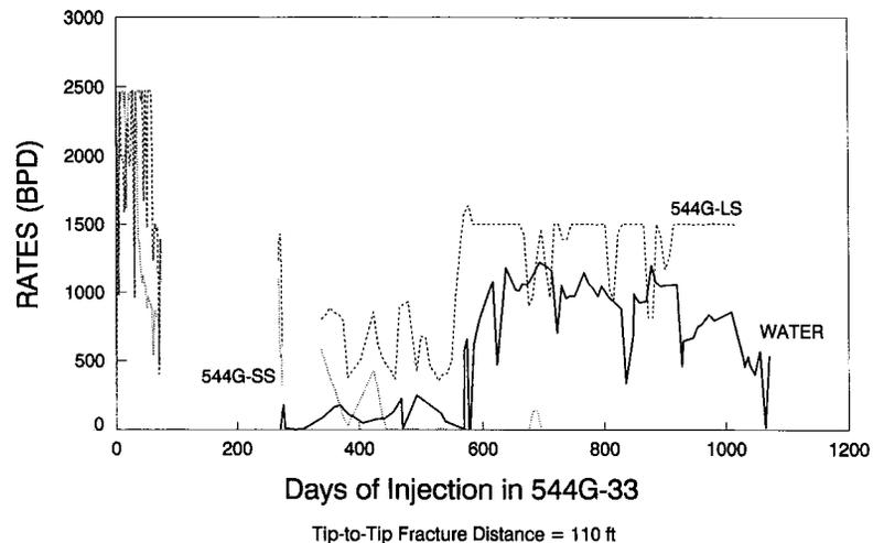
Fig. 16—Phase B producer 543S-33 links with the long injection string of the dual injector 544G-33. The production rate is limited by the pump-lift capacity.
