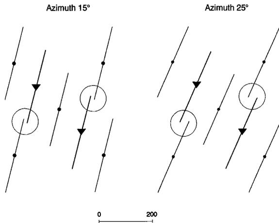
Fig. 7—Injector-producer linkage in the ¼-acre (0.5-ha) staggered line waterflood pattern; the assumed half-length of hydro-fractures is 135 ft (41 m).
