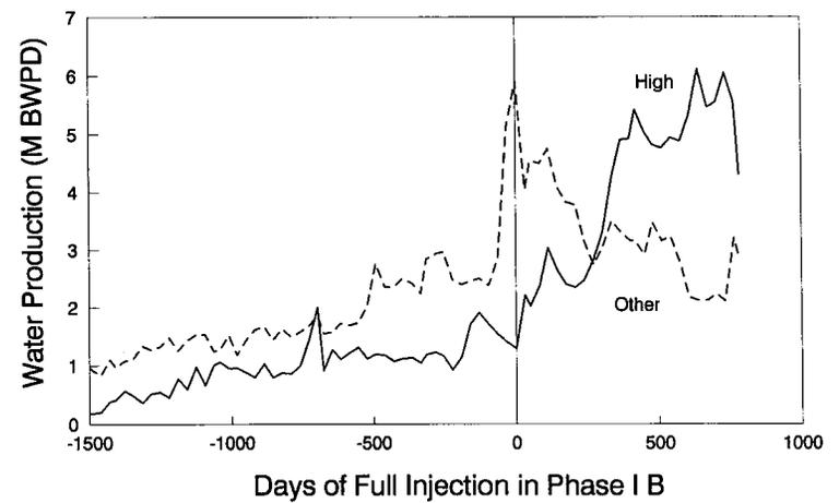
Fig. 12—Water production rates for "High Gross" and "Other" wells in the Phase I waterflood. Note that water production in the "High Gross" category kept on increasing until the injection rates were curtailed. In contrast the "Other" category rate declined as the square root of time. Note a dramatic increase of water production after 180 days of injection.
