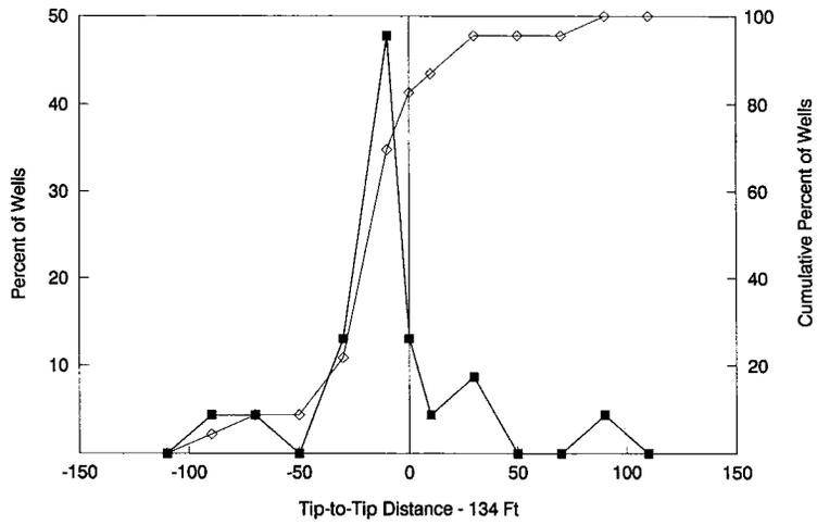
Fig. 5—The distribution of tip-to-tip distances between a producer hydro-fracture and that of an injector NE or SW from the producer for all the Phase IA producers (assumed fracture half-lengths and azimuths are 125 ft (38 m) and N15°E, respectively).
