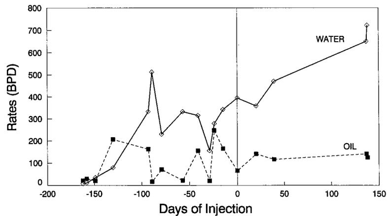
Fig. 19—Oil and water production rates in Well 531E1-33 that first linked with injector 531L-33 and then 538A-28. Note that no production tests were performed between 40 and 140 days.
