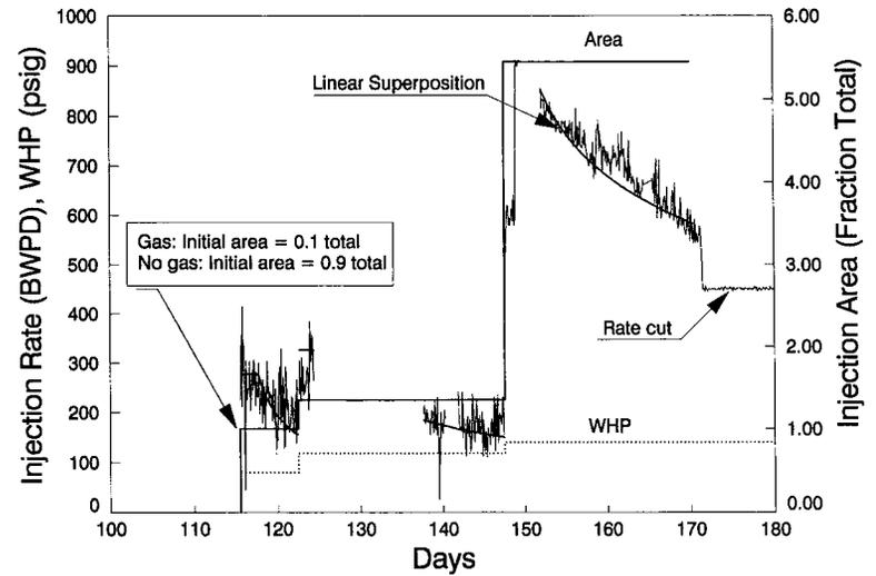
Fig. 25—Injection rate and fracture extensions during two pressure steps in Phase IIIA injector 537E-34. Note that in the worst case the fractures could grow up to five times the design area.
