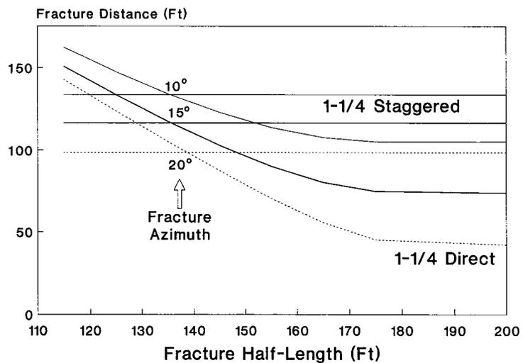
Fig. 3a—Fracture-fracture distance vs. fracture half-length for 1¼-acre (0.5-ha) direct and staggered line patterns.
