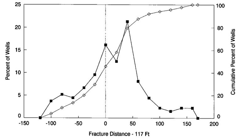
Fig. 6—The distribution of plane-to-plane distances between a producer hydro-fracture and that of an injector NE and SW from the producer for all the Phase IB producers (assumed fracture half-lengths and azimuths are 125 ft (38 m) and N15°E, respectively).
