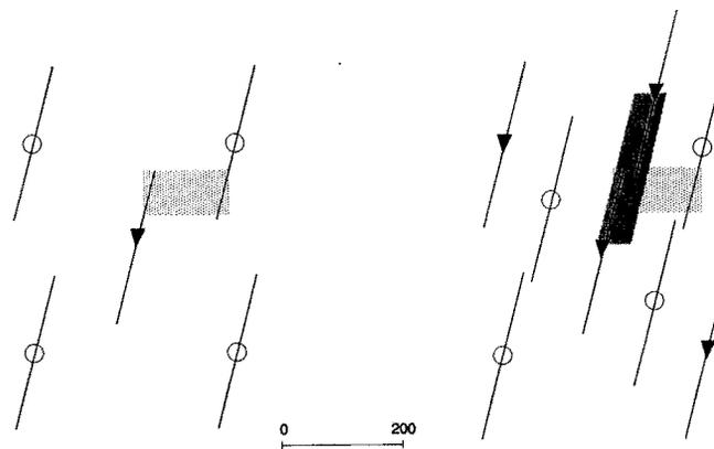
Fig. 23—Producer-injector coupling on 1 ¼-acre spacing may preclude a future ¼-acre development.
