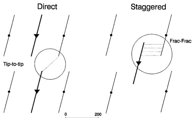
Fig. 2—How hydro-fractures may link in 1¼-acre (0.5-ha) direct and staggered line waterflood patterns. The assumed half-length and azimuth of the fractures is 135 ft (41 m) and N15°E, respectively.
