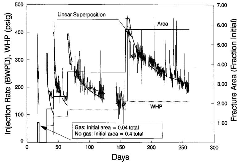
Fig. 26—Injection rate and fracture extensions during four pressure steps in seven-pattern, 1/4-acre waterflood pilot injector 531A1-33. Note that in the worst case the fracture area could be twice the design area.
