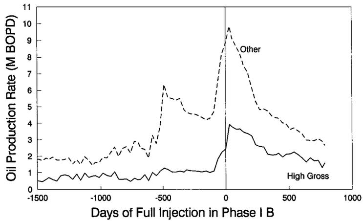
Fig. 11—Oil production rates for "High Gross" and "Other" wells in the Phase I waterflood. Note a steeper rate of decline in the "Other" category.
