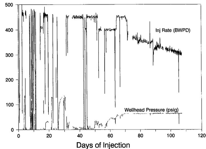
Fig. 20—Injector 531L-33 links with 531E1-33 and pressures up after 70 days of injection.
