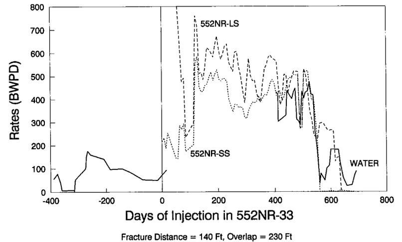
Fig. 14—Phase IB producer 522NR-33 links with the long injection string of the dual injector 552-33 and free flows.
