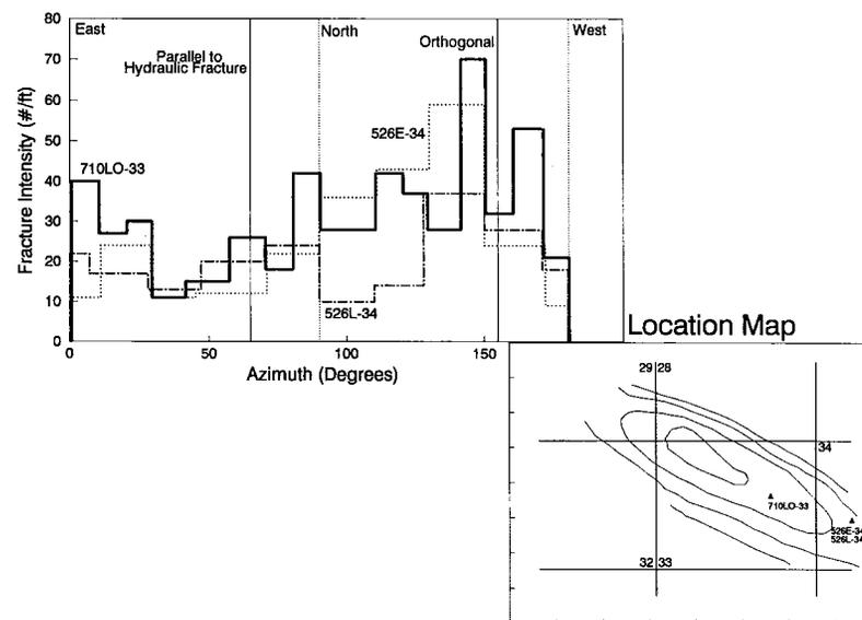
Fig. 4—Intensity of natural fractures vs. their azimuths (from oriented cores in the Diatomite Wells 526E-34, 526L-34, and 710LO-33).
