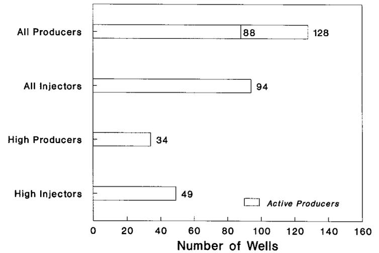
Fig. 8—Classification of wells in the Phase I waterflood (Section 33).
