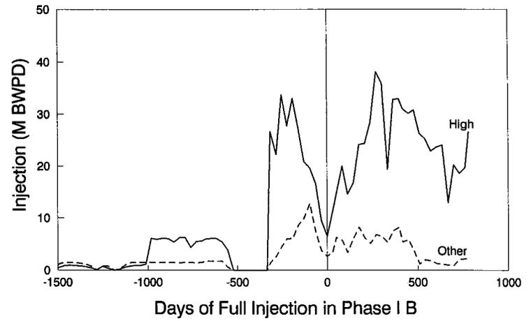
Fig. 10—Injection rate of water for the "High Rate" and "Other" Phase I waterflood injectors.
